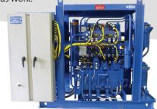
UNIT: Steel Casting Valve Rack PRIMARY FLOW: Approximately 300 GPM WORKING PRESSURE: 2,000 - 3,000 PSI PURPOSE: This valve stand modulates the flow of molten steel during the steel casting process
