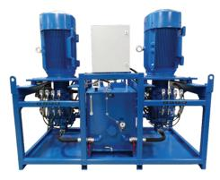
UNIT: Shredder COMBINED PRIMARY FLOW: 320 GPM WORKING PRESSURE: 5,000 PSI PURPOSE: This closed-loop system powers a material shredder for process testing of various materials.
